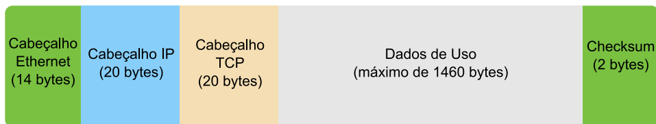
FIGURA 20.2 PACOTE ETHERNET TCP/IP
